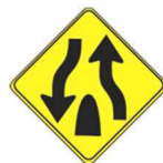
Divided Highway Ends
